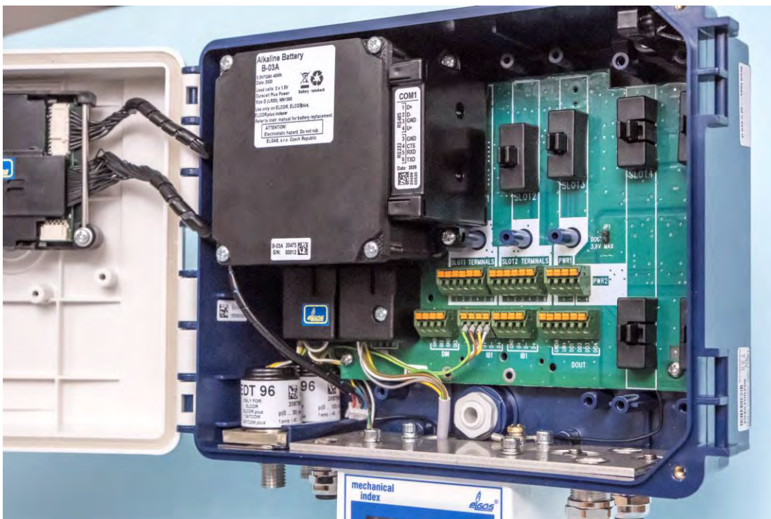
Fig. 42 ELCORplus indexer with alkaline battery B-03A located above slot 0
