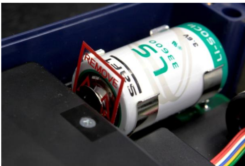
Fig. 19 Removable foil strip at battery holder
