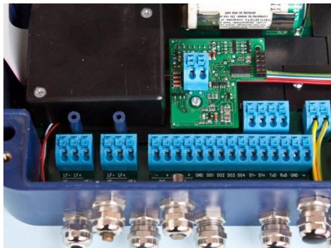
Fig. 11 Encoder SCR board (without cover)
