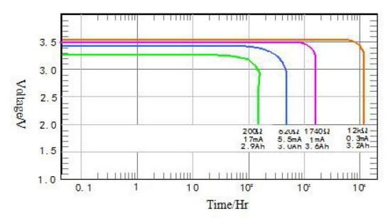
Different discharge current and discharge capacity characteristics
