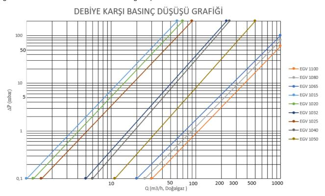
Flow Conversion: The above flow values and flow capacity table are prepared for natural gas. If our gas valves are used in a gas other than natural gas, the flow of the other gas is found according to the flow conversion formula below.
